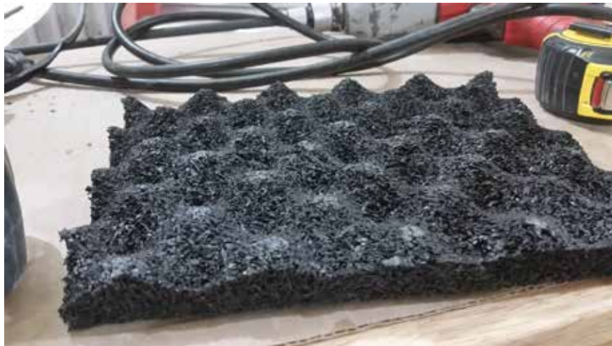
Figure 4 – Sample of composite flooring layer 1
