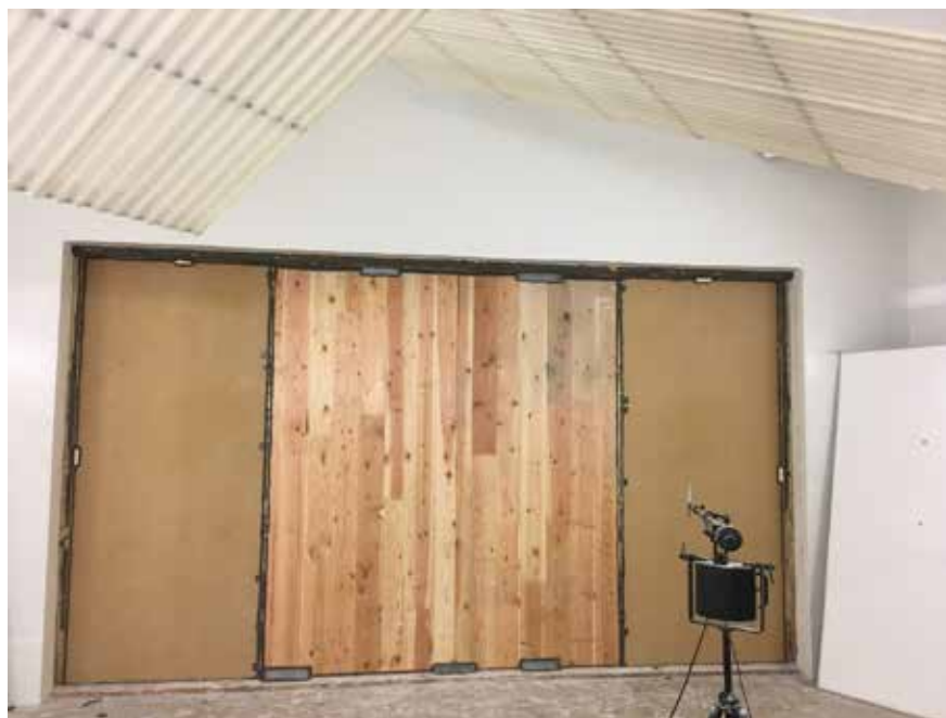
Figure 1: Specimen prior to addition of insulation and cedar siding
