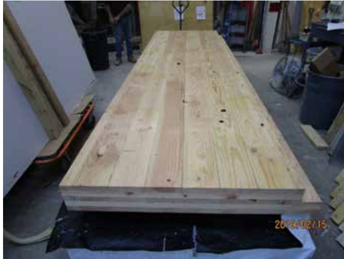
Figure 3 – Individual cross-laminated timber panel
