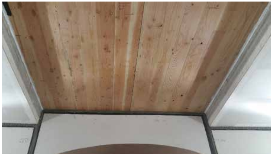
Figure 2 – Underside of installed test specimen, as viewed from receive room
