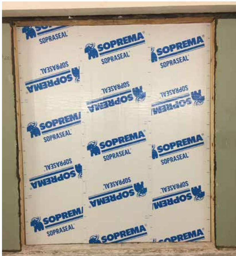
Figure 3: Specimen with membrane
