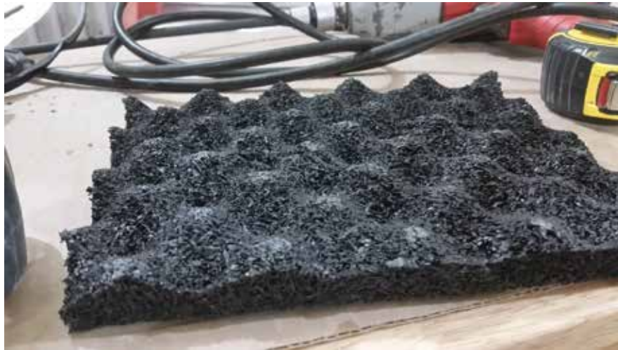
Figure 4 – Detail of bonded crumb rubber underlayment
