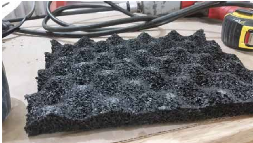
Figure 4 – Detail of bonded crumb rubber underlayment
