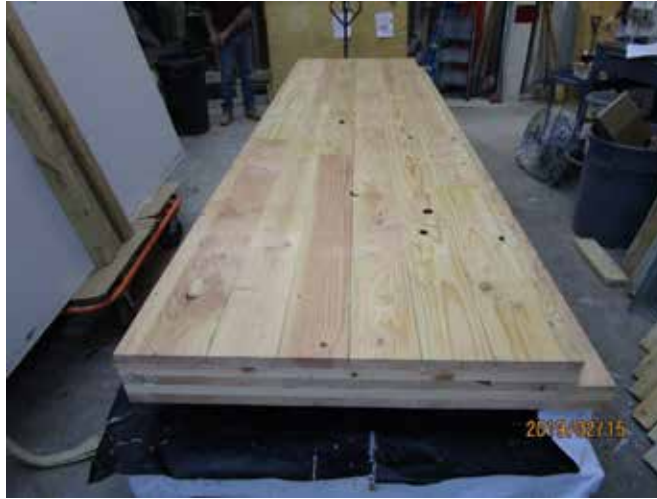
Figure 3 – Individual cross-laminated timber panel
