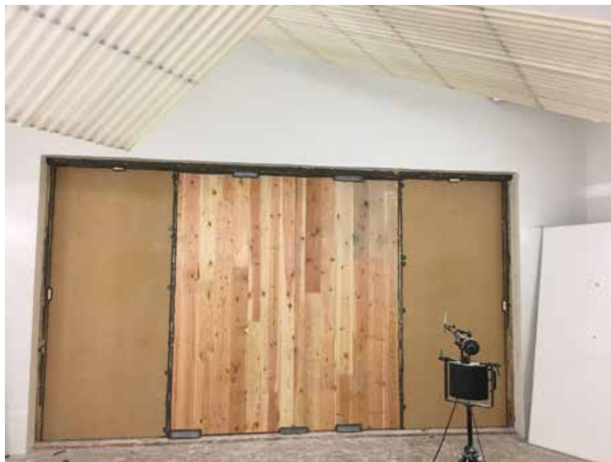
Figure 1: Specimen prior to addition of gypsum wall board
