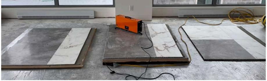
Left: Different underlayments options laid out in a controlled environment, Top Right: Overview of the testing setup, with technicians ensuring precise installation Top Left: Acoustic testing of the different underlayments
