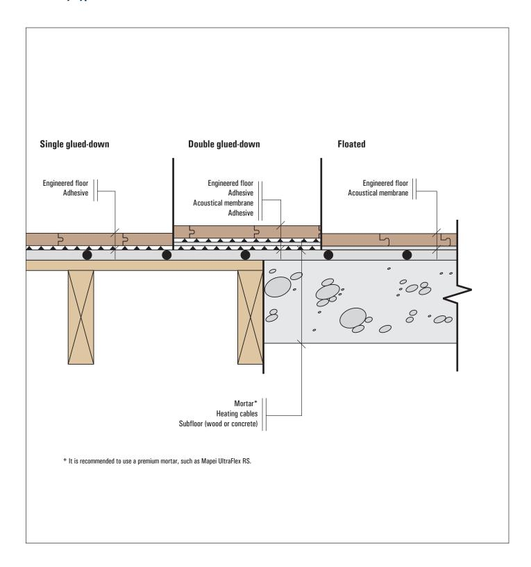
2.2 Installation method with self-levelling compound
