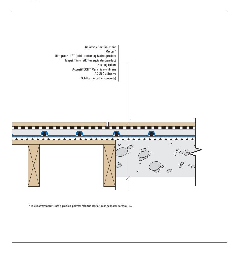
2.1 Installation method with trowel and mortar, cables under the membrane
