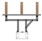
**2.** RSIC™ Garage Rail Isolation Kit Includes isolators for mounting the garage door rails
