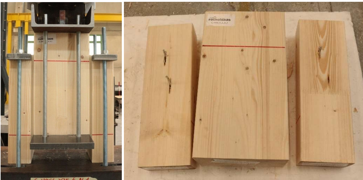
Figure 7 Observed failure mode at the end of the cyclic test.
