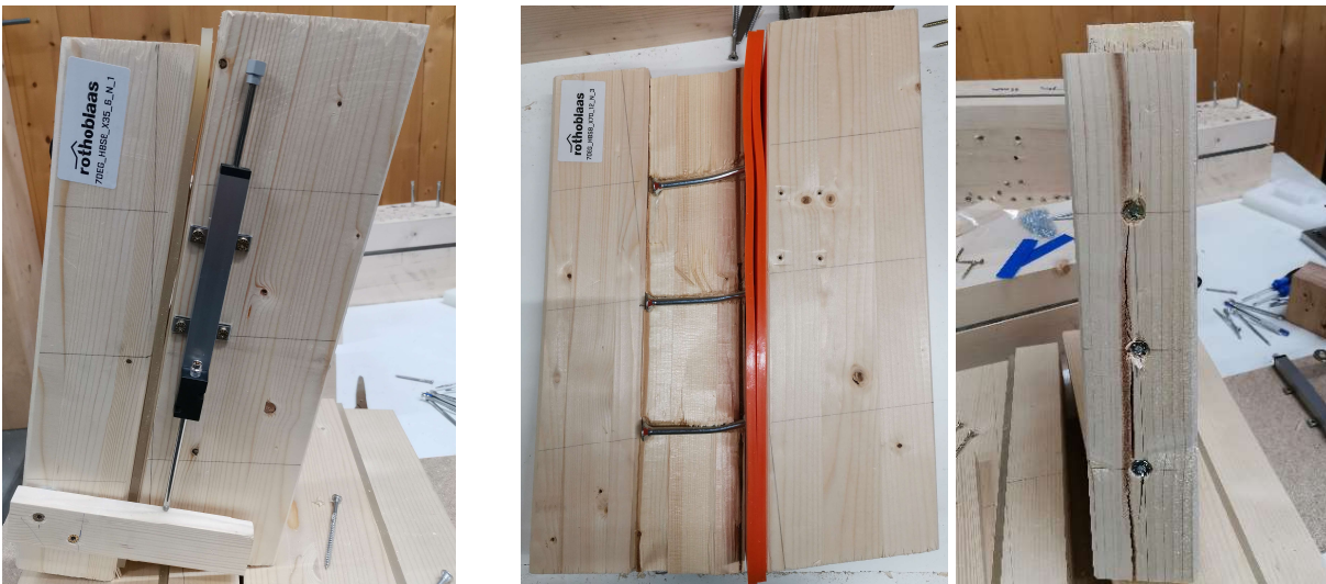
Figure 4 Observed failure mode at the end of the monotonic tests.
